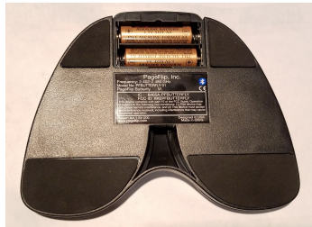
Figure 2: Battery cover is located at the bottom of the PageFlip Butterfly.
